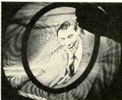
Before you do any setup adjustments in a color-TV set, always degauss the CRT, chassis and cabinet if it is metal.
