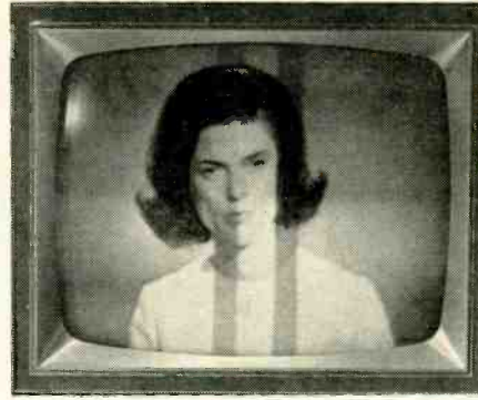
How tuning bars look on the screen. The single bar indicates optimum tuning. In right-hand photo movable bar is on the right. Fine-tuner should be rotated counterclockwise.
