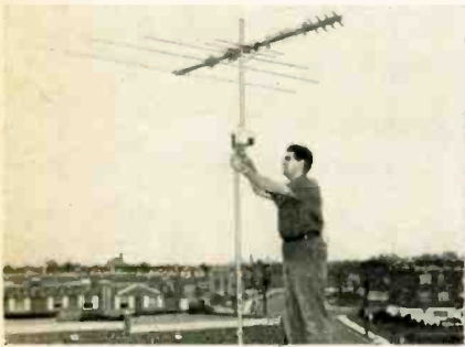
One way to minimize ghosts—use a flat-response directional antenna with a rotator. Then aim for the best picture.
